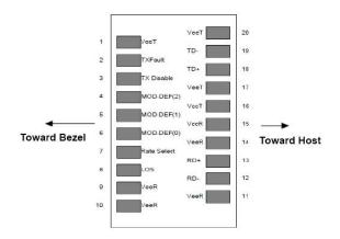
**Pinout of Connector Block on Host Board**
